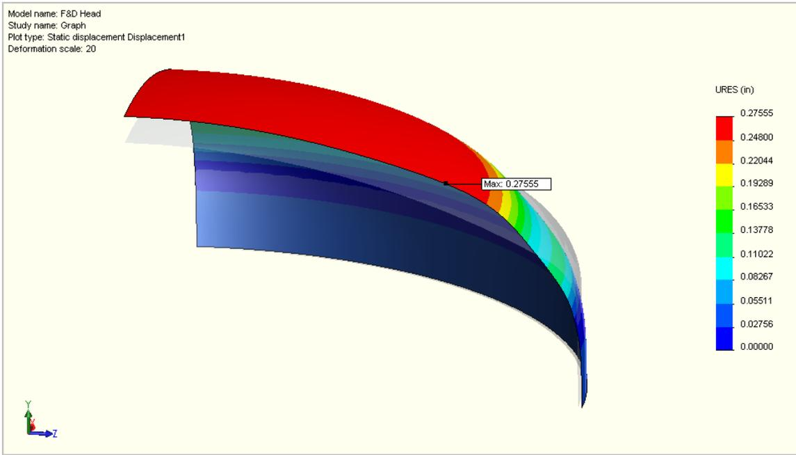
The complete F&D head has a maximum displacement is 0.277” much higher than previously found in the individual components. Each component does not displace uniformly as shown in the previous studies.
