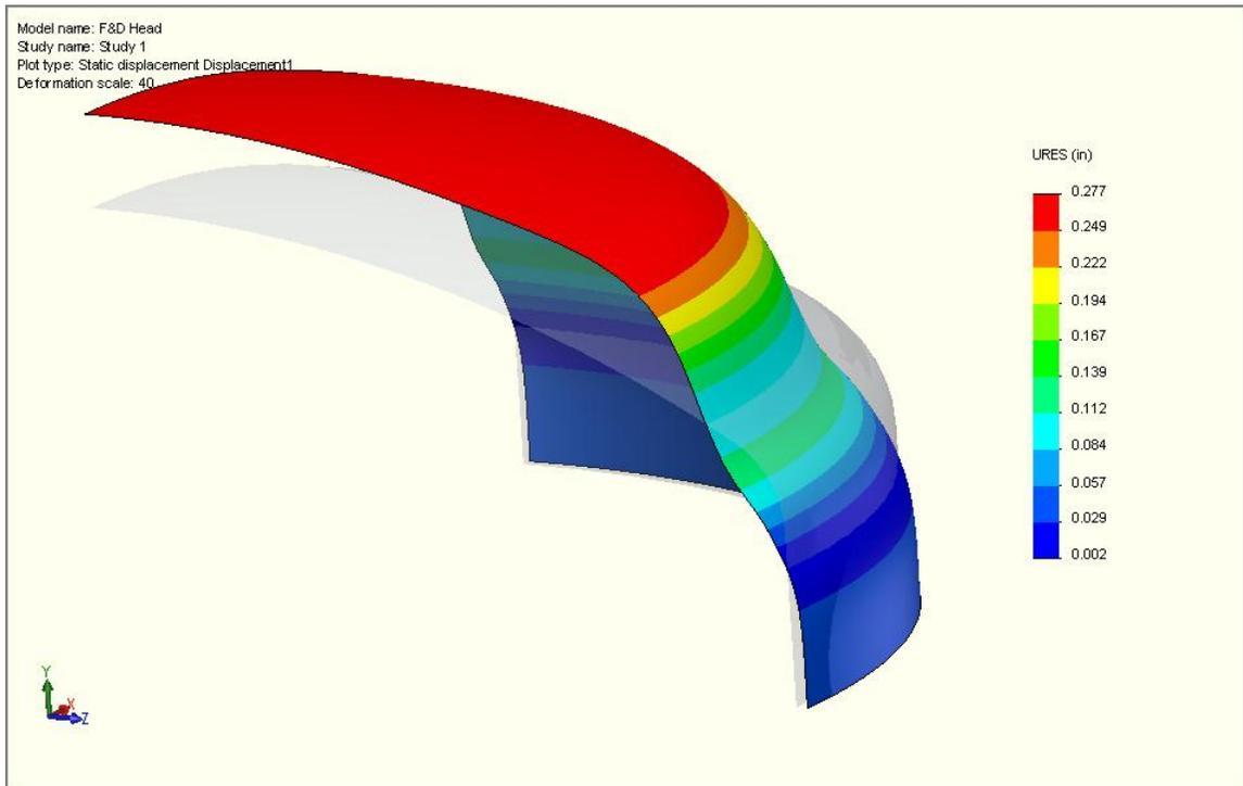
An exaggerated view of the F&D head's displacement shows that the knuckle pushes inward as the crown and straight section deform radially outwards.
