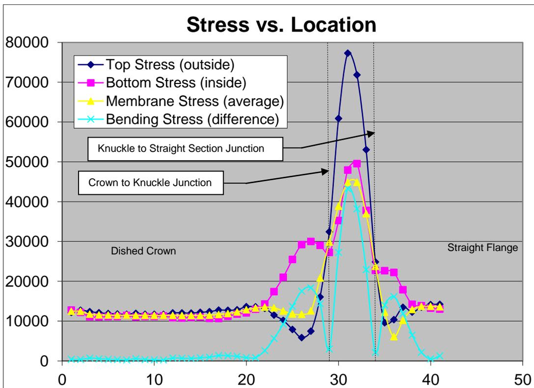
This F&D head designed to the VIII-1 rule UG-32 has stress in excess of the amounts allowed in VIII-1 Section UG-23. If F&D heads were invented today we would put a lower allowed pressure rating on them than UG-32 provides, however we have 100 years of experience that indicates that higher stresses can be used in this case.
