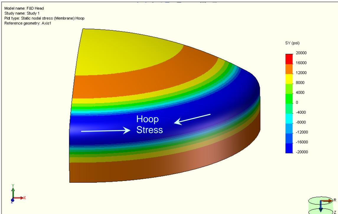
The displacement plot shows the knuckle pushing inward. The hoop stress plot shows the region of compressive stress at the knuckle.
