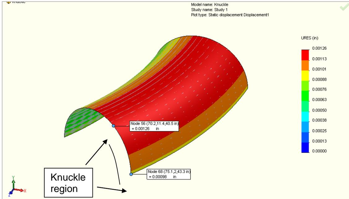
The knuckle is a section of a torus. The maximum displacement is 0.00126", found at the point where the knuckle meets the crown. Results have also been probed at the point which meets the head straight section.
