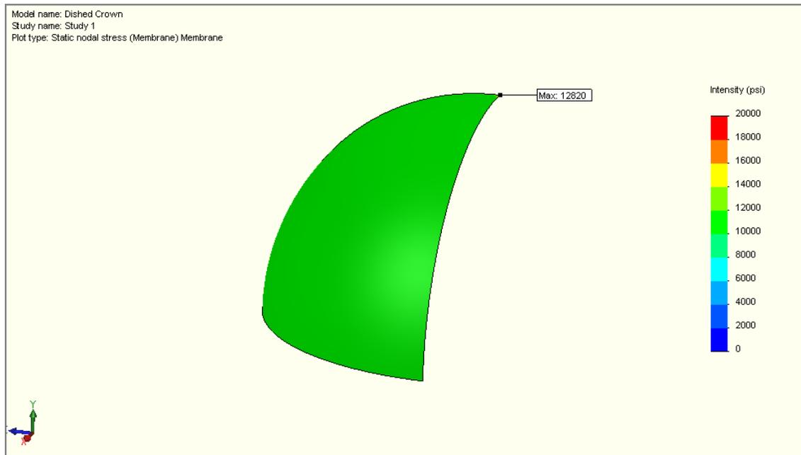
The membrane stresses in the crown are a uniform 12,820 psi - less than the allowable 20,000 psi.
