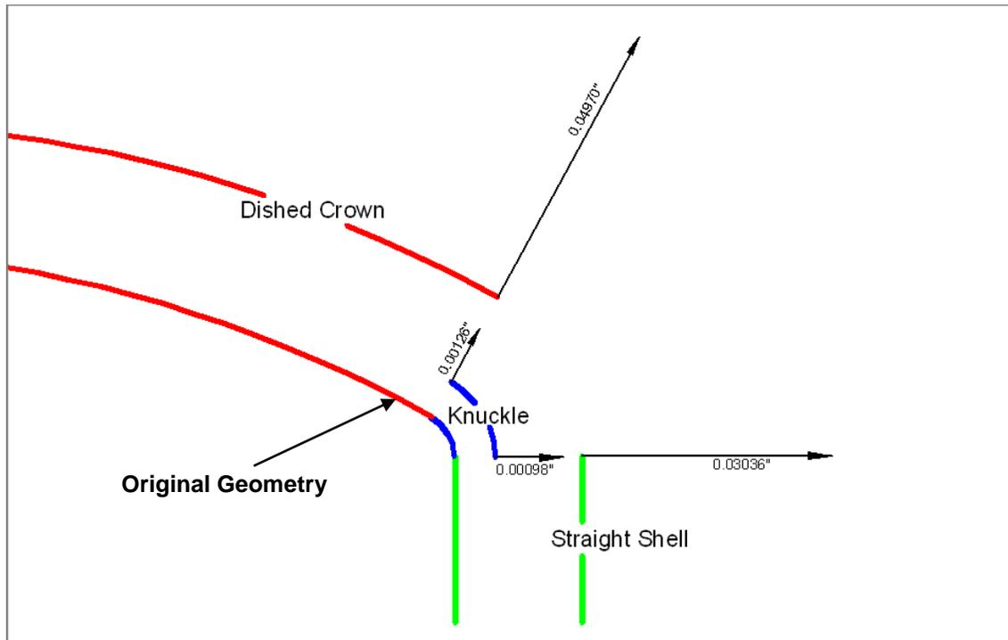
The resulting displacement vectors of each separate head component. The displacements of adjacent components are not equal. This is the source of the high computed stress.
