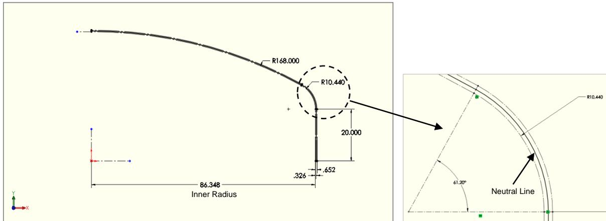
The above image shows all geometry of the F&D head. Note that all dimensions are referenced to the inside surface of the head, however the shell model is created from the neutral line running half way between the inside and outside surfaces.
