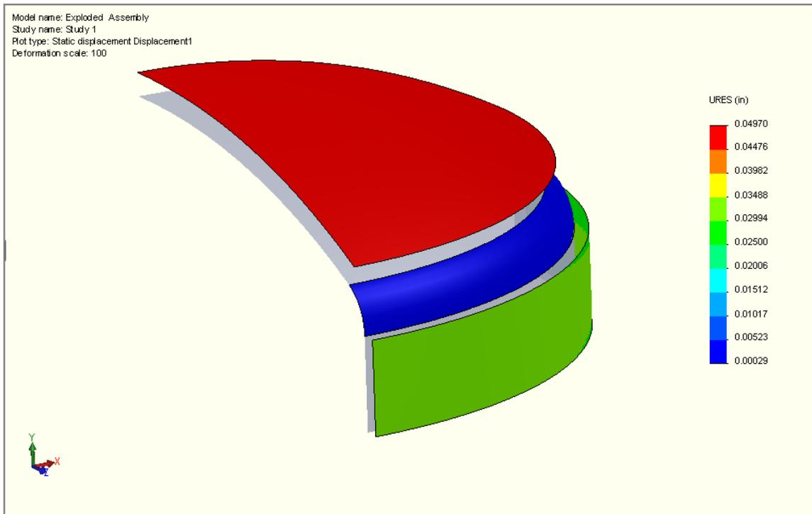
The dished crown and straight flange section need a much greater displacement than the knuckle.
