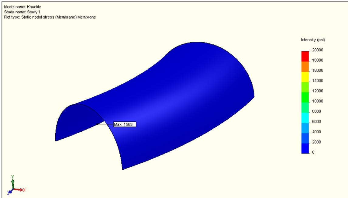
The Membrane Stresses is relatively uniform. The maximum stress is 1583 psi which is below the 20,000 psi allowable.
