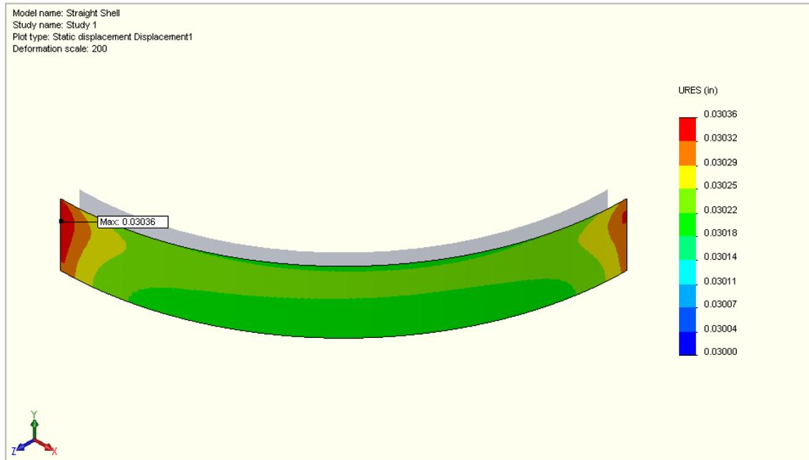
The above image shows a section of the straight pipe component of the head. The displacement in the straight pipe model is relatively uniform. The maximum displacement is 0.0304”.
