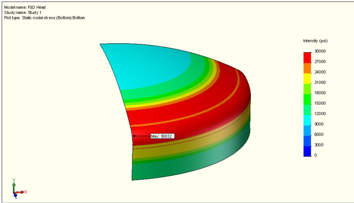
The top side stress (bending + membrane) is far above the 20,000 psi VIII-1 basic material allowable.
