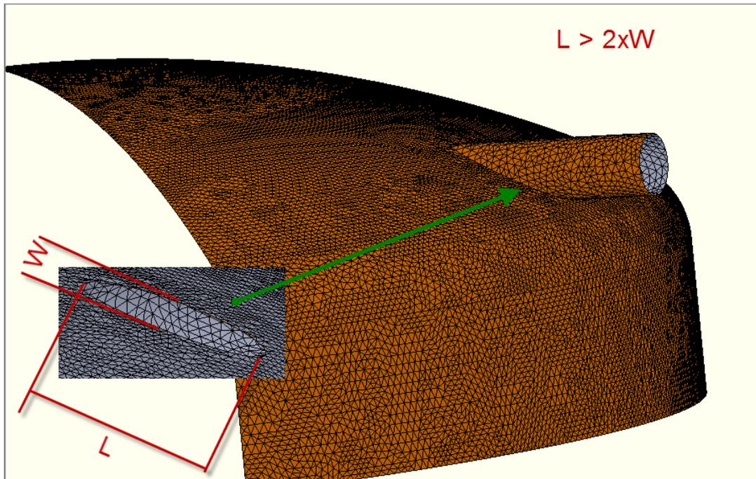
The simple solution was to relocate the nozzle into the much lower stressed crown area, and have the pipe come in at an angle so that the opening would be less than 2x long to wide. The project could then be finished using regular code rules.
