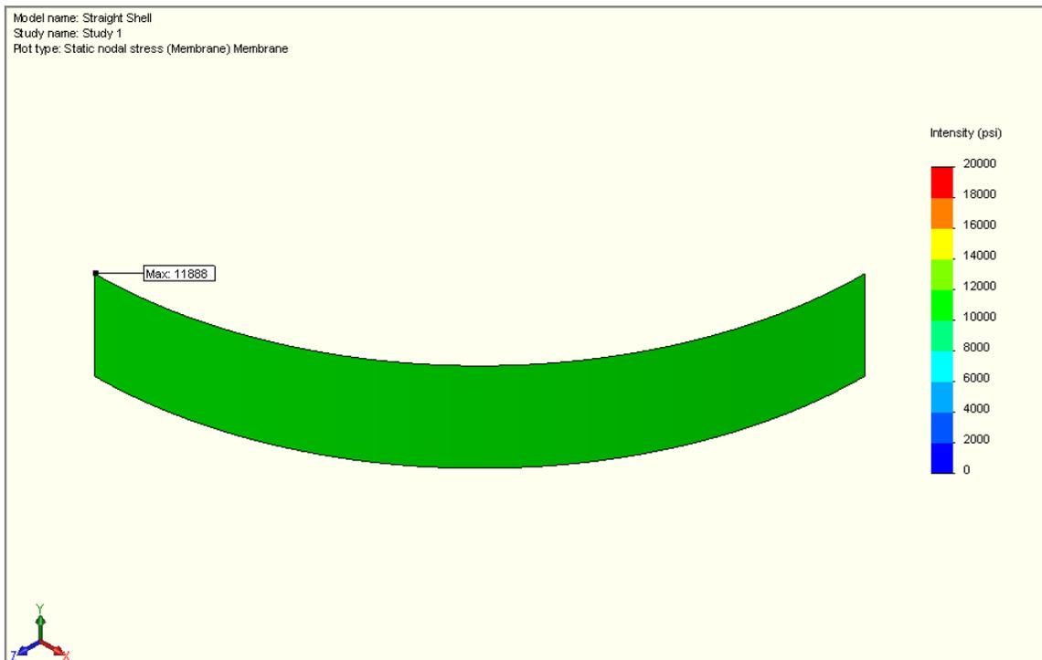
The above image shows the Membrane Stresses in the straight pipe model section. The stress is uniform. The maximum stress is 11,765 psi which is below the 20,000 psi membrane allowable.
