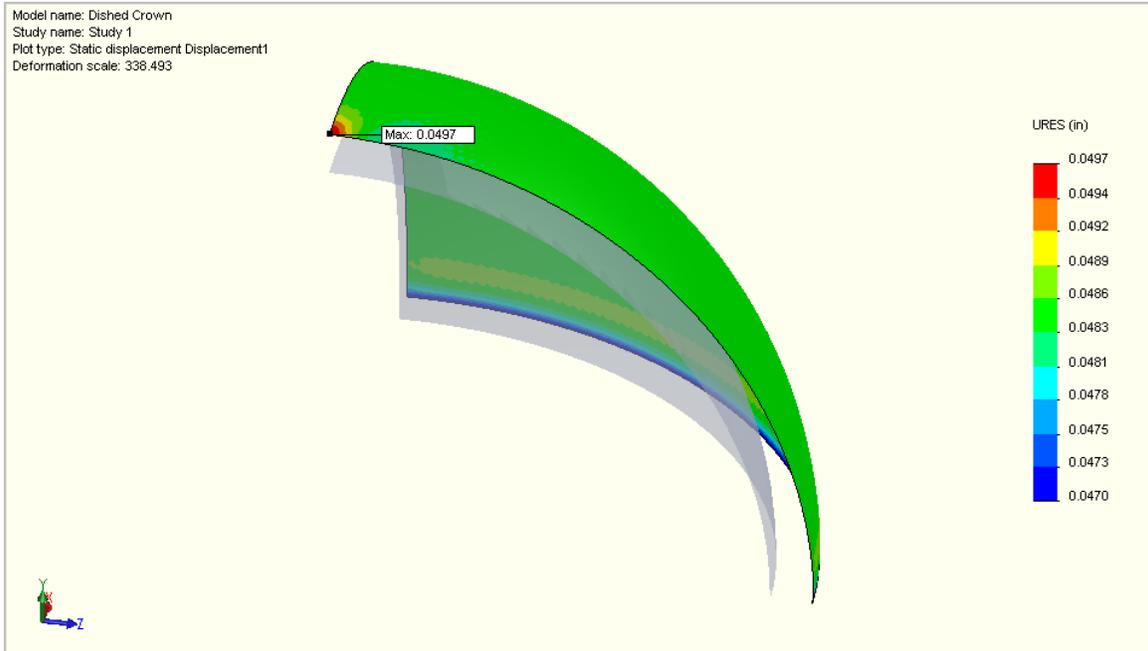
The crown on its own displaces as if it is part of a radially expanding spherical shell. The average displacement is 0.0483”.
